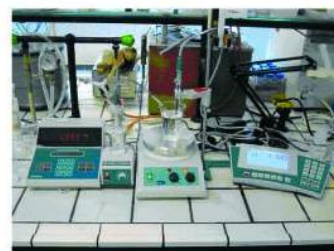
IEC 60754-2 Gas Acidity Test
