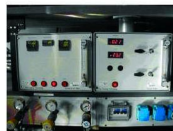
ISO 4589-2 Oxygen Index Test
