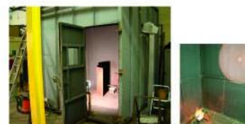
IEC 61034 Smoke Density Test
